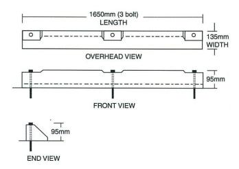
Replas wheel stops are easily handled by one person. Suitable for installation in any hard surface parking area, they prevent contact with walls, garden beds, pathways and other vehicles. Fixings are
